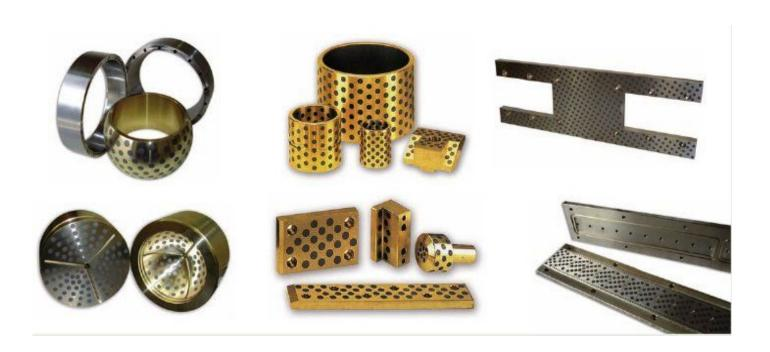
The **INSERTS IN GRAPHITE** are distributed over 20-30% of the running surface, creating an anti-friction thin film that will remain during the rest and is under heavy loads. On request could may be applied a film of 20 um of composition similar to that of the insert to facilitate the early movements and avoid a damaging blow to departure (stick-slip).
